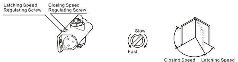
**BACK-CHECK ADJUSTMENT** — is controlled by the adjustment valve, BACK-CHECK is now set for soft action. To INCREASE Back-check action turn valve CLOCKWISE. To DECREASE, or to TURN OFF Backcheck action turn valve COUNTER CLOCKWISE.
